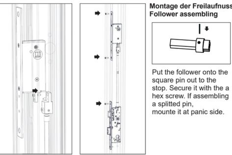
The door selector is pushed onto the connector and screwed in place via the upper small forend hole using an allen wrench 2.5 AF. Here, the pin on the connector acts as a guide.
