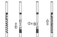
All shot bolts must be mounted securely in the connecting piece of the lock. Only the upper shot bolt rod (systeQ 9650) can be rotated slightly out of the connecting piece of the lock for adjustment purposes without compromising its function.
